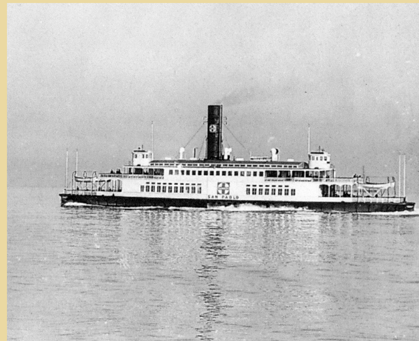
The ferryboat San Pablo operated at Ferry Point from 1900 until 1933. Custom-built for Santa Fe by Union Iron Works in San Francisco, the ship originally burned coal, but was later converted to oil. It measured 226' by 36' and its engine drove two 16' paddle wheels.
