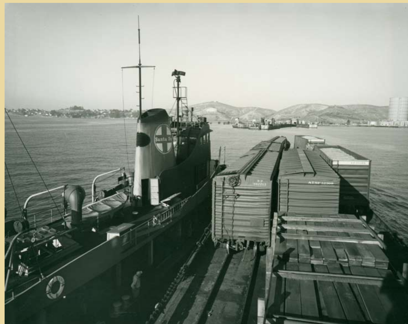
The Santa Fe tugboat Edward Engel nudging a freight barge toward the Ferry Point wharves. The 250' long barges held 14-16 railcars each, and had a draft of 6' when fully loaded.
